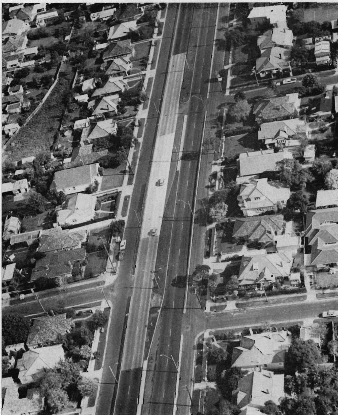
Plate 3—Experimental seal using calcined pyrophyllite synthetic aggregate. Aerial view of test sections on the west-bound carriageway of North Road, Ormond. From bottom to top the sections are (a) older basalt seal, (b) newer basalt/calcined pyrophyllite (2:1 ratio) seal, (c) calcined pyrophyllite seal, (d) scoria/calcined pyrophyllite (2:1 ratio) seal, (e) old asphalt surfacing.
