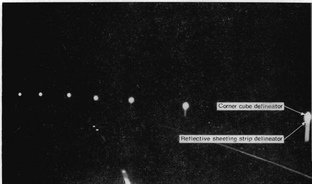
Plate 5—Night view of guide-posts, showing the relative performances of corner-cube delineators and reflective sheeting strip delineators. It will be noted that the former appear far larger and brighter than the latter.
