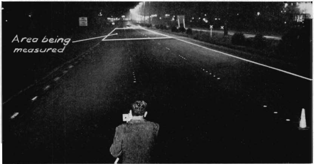
Plate 6—Rosenhagen road luminance meter in use to determine the average luminance of the area shown. The 1^\circ observation angle between the instrument and the road at the centre of the observed area is approximately equal to the angle between a car driver's line of vision and the road.
