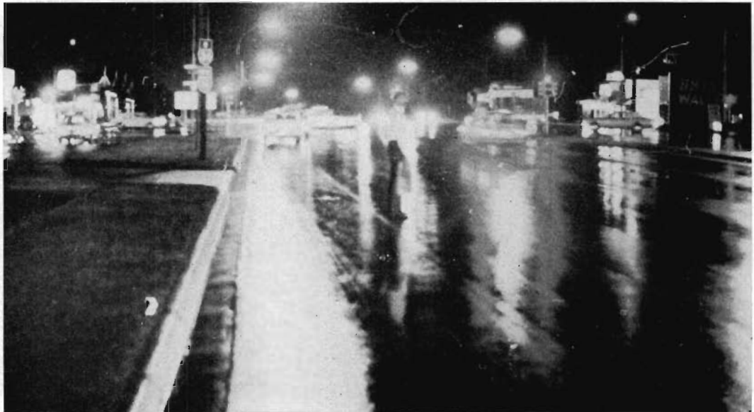
Plate 11—Pedestrian scarcely visible, due to light reflections, when standing on a smooth asphalt pavement on the Maroondah Highway. This pavement is adjacent to that shown in Plate 10 and the conditions of weather and lighting were the same in each case.
