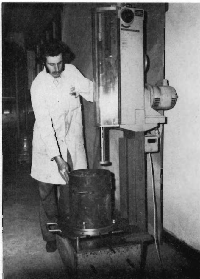
Plate 16—Modified Farnell compaction machine for compacting 3 in. maximum size material.
