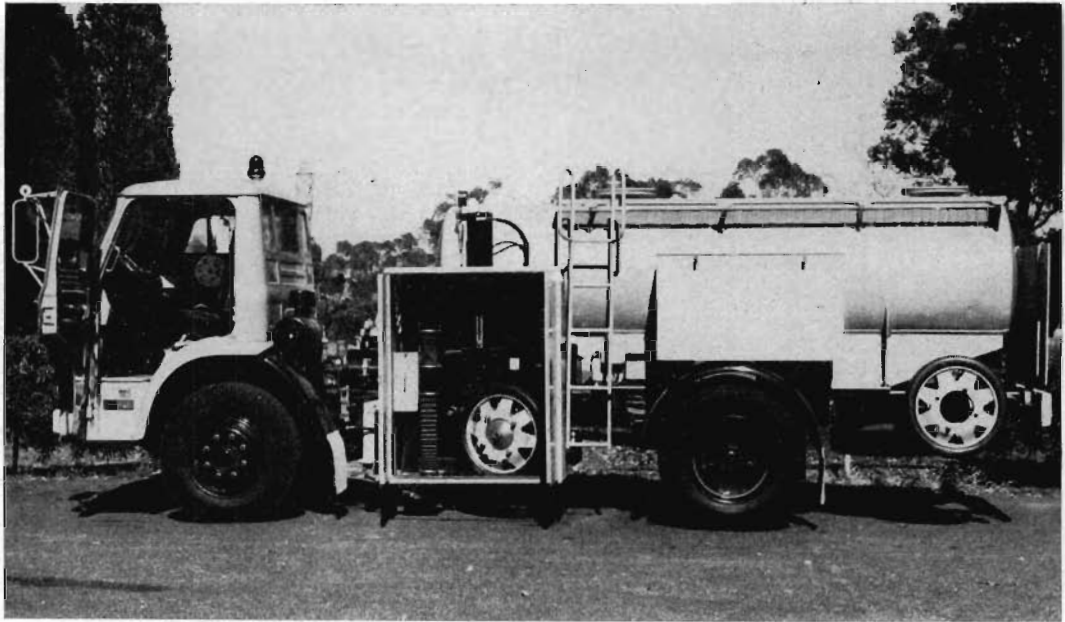
Plate 13—Sideways-force Coefficient Routine Investigation Machine (SCRIM) with inclined test wheel in non-operating position behind the cab and spare test wheel attached at rear of vehicle.
