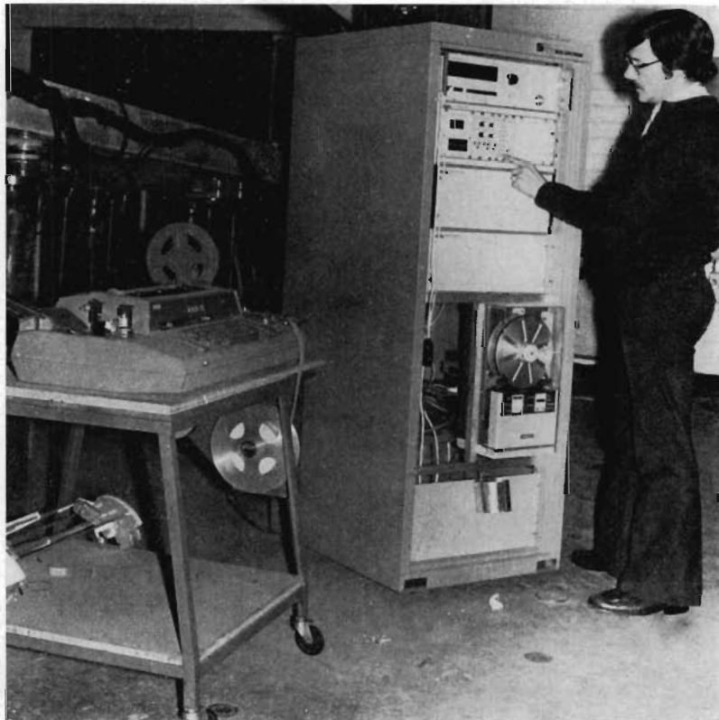
Plate 3—Data acquisition system recording data from the 1/10th scale model of Gordon Street Overpass.
