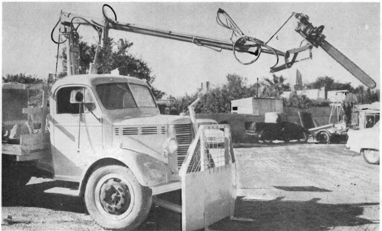
Plate 3.—Tree lopping unit, showing the hydraulic linkage and electrically operated chain saw.
