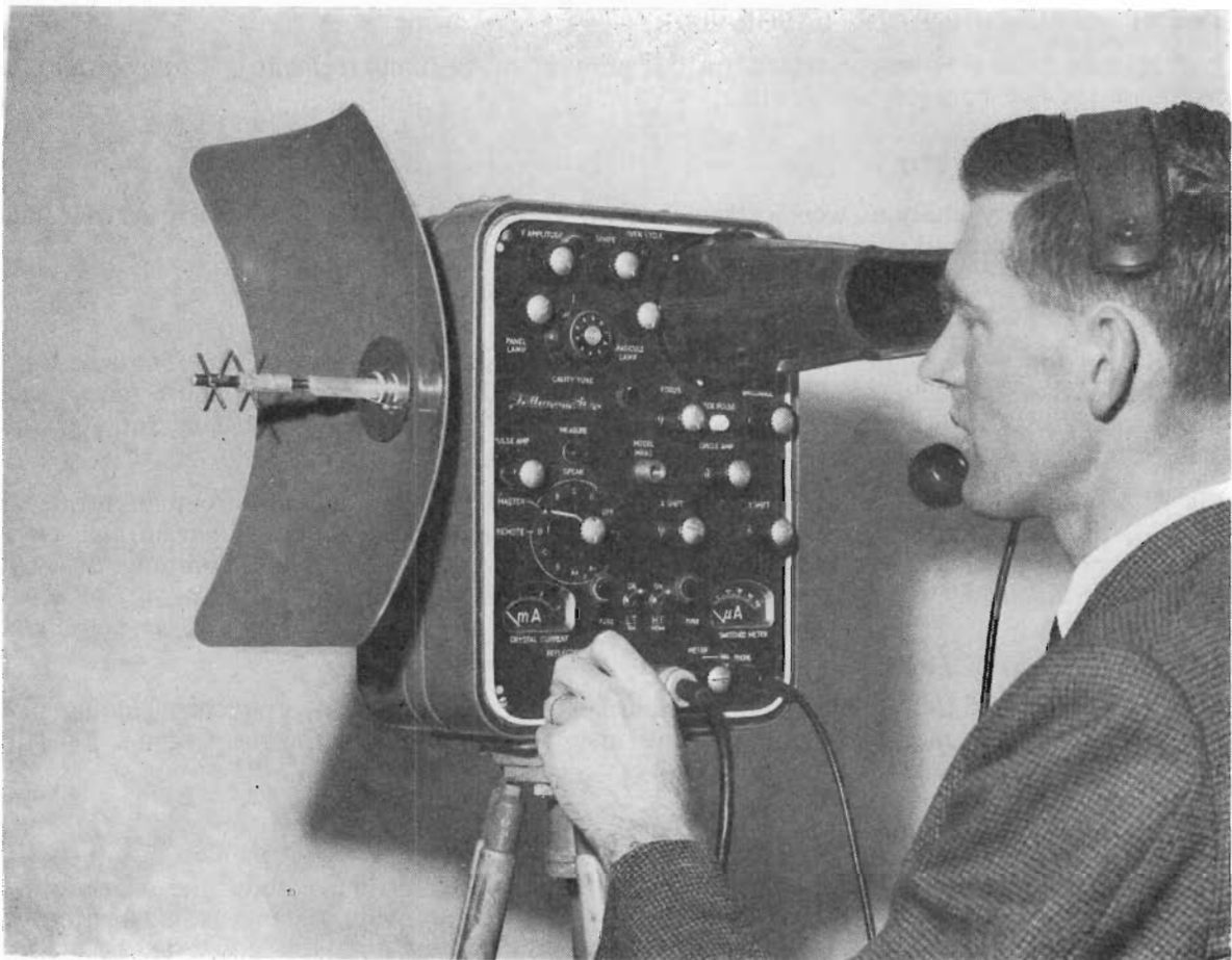
The tellurometer measures distances by the time of reflected radio waves between two such instruments. The system is accurate to about 6 inches in 20 miles. * * * *
