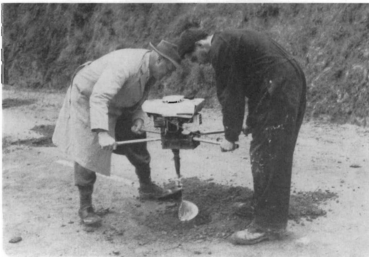
Plate 1—Motorized Two-man Posthole Auger in Operation
