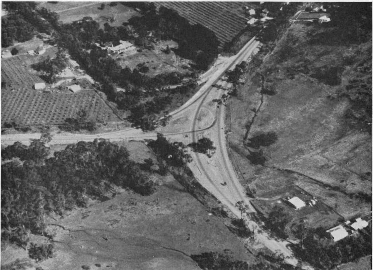
Plate 21.—Maroondah Highway. Channelization at intersection of Maroondah Highway and Warburton Highway, near Lilydale.
