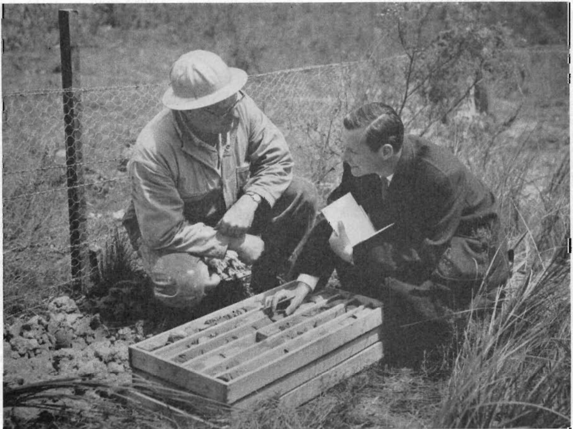
At Devilbend Project, samples of rock extracted by a diamond drill are being examined and logged.
