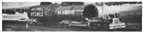
Plate 45.—Fractionator 135 feet long, 16 feet wide, en route Melbourne to Adelaide. Gross weight 98 tons.
