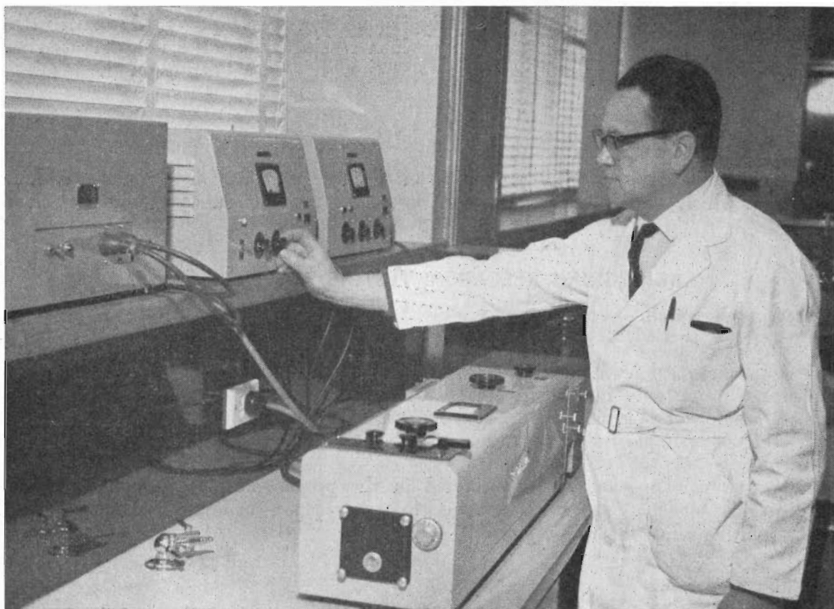
A special water test being carried out in the Commission's Engineering Laboratory with the spectrophotometer.
