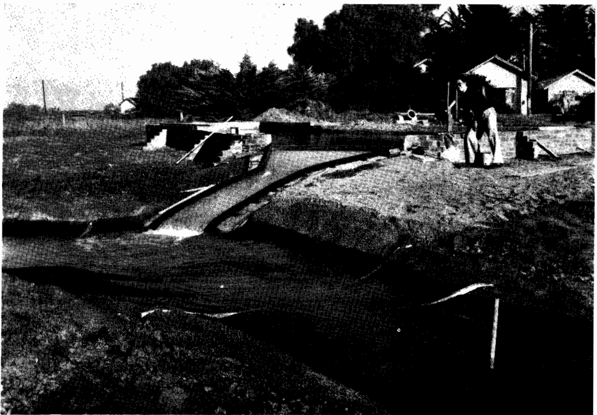
Model of the spillway for Eppalock Reservoir, now under construction. Models such as this provide essential data for the Commission's engineers.
