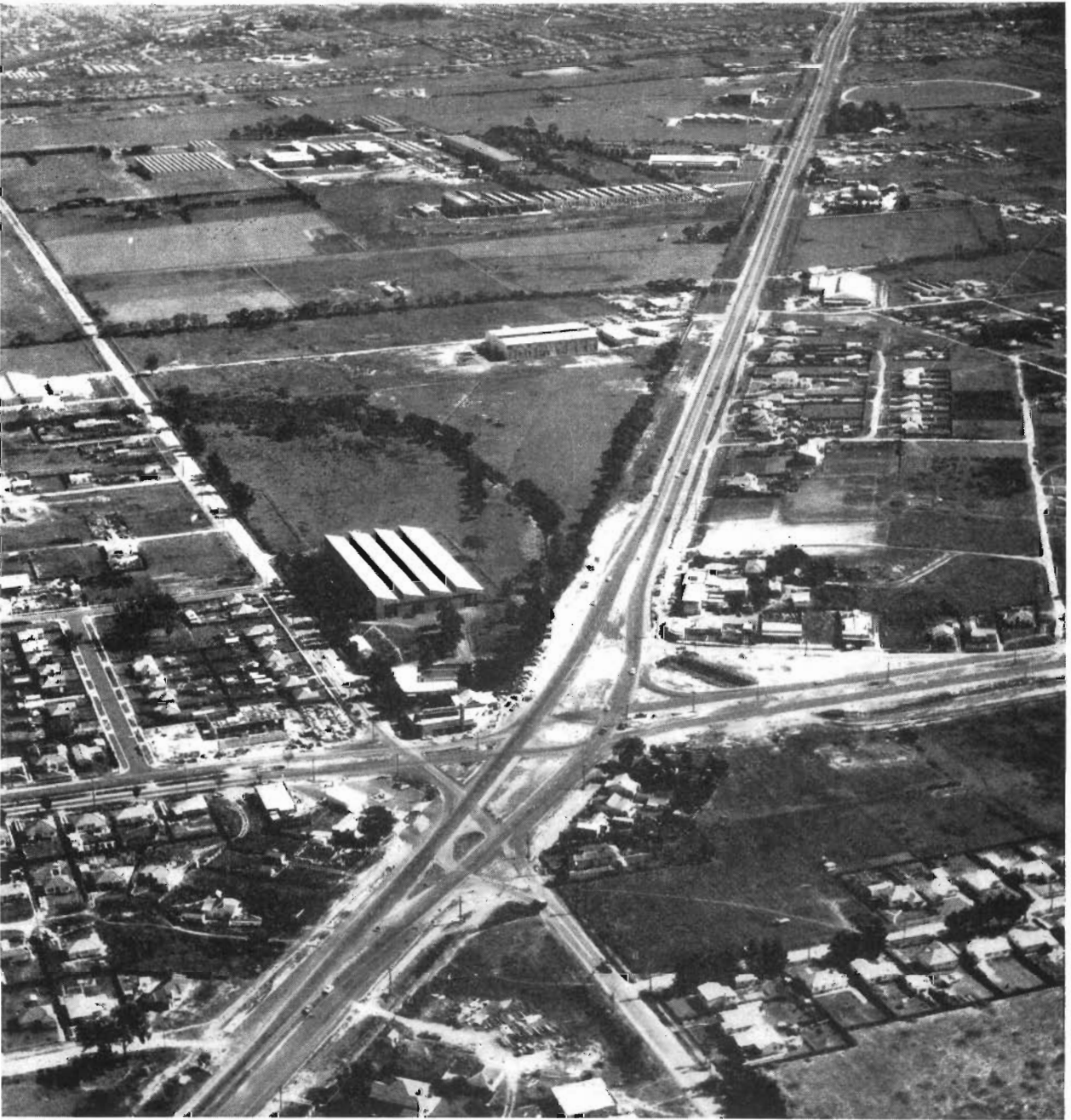
Plate 11.—Princes Highway East at Springvale. Duplication of pavement between Oakleigh and Dandenong. Channelization at intersection with Springvale main road, Centre Road, and Police Road.
