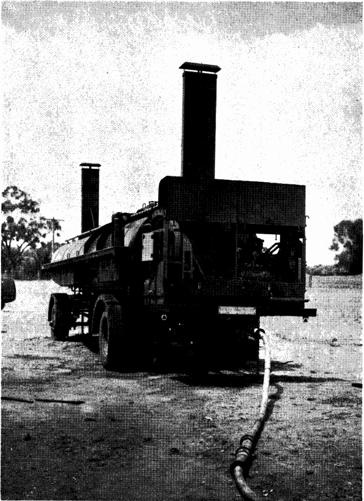
Fig. 6.—Heater-storage tanker pumping into sprayer.
