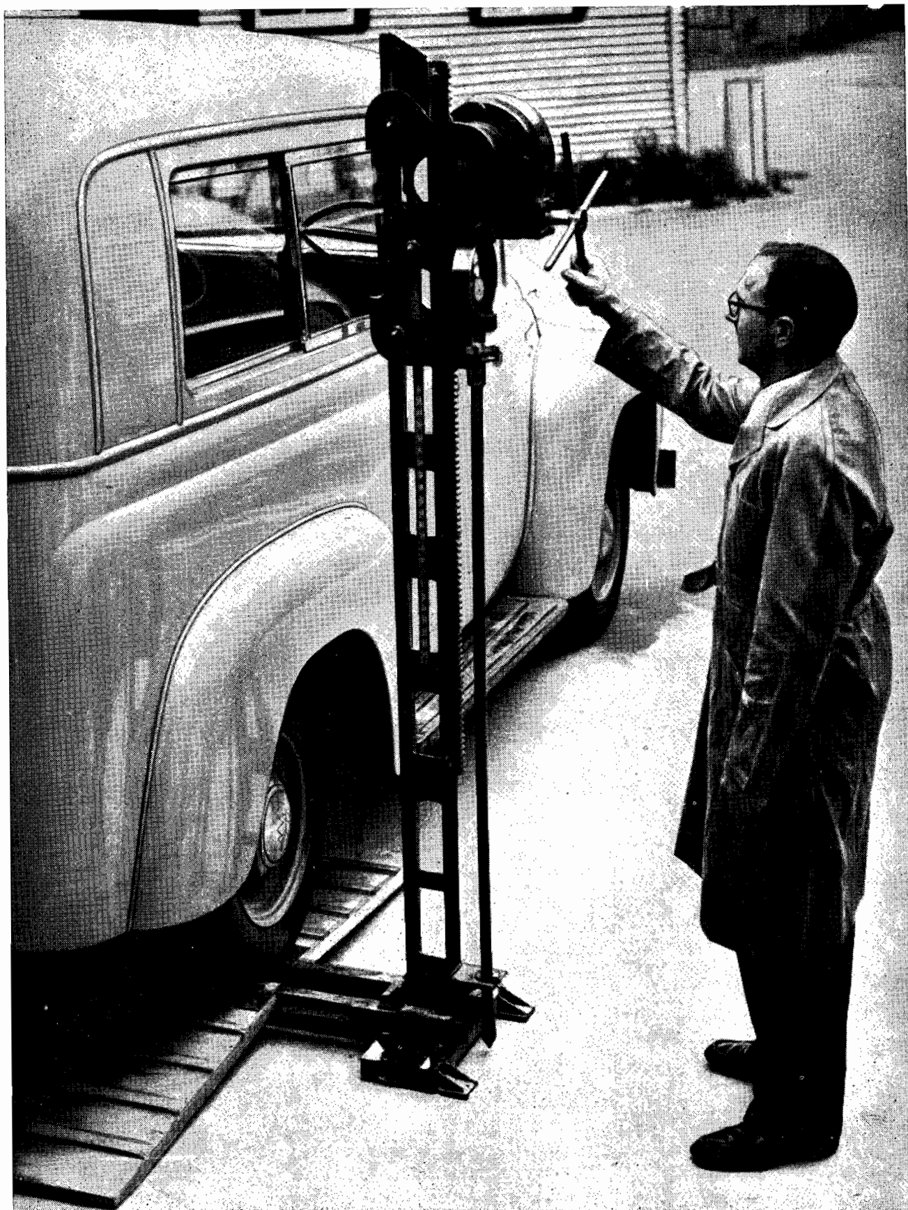
Fig. 9. Static cone penetrometer set up as for use in the field.
