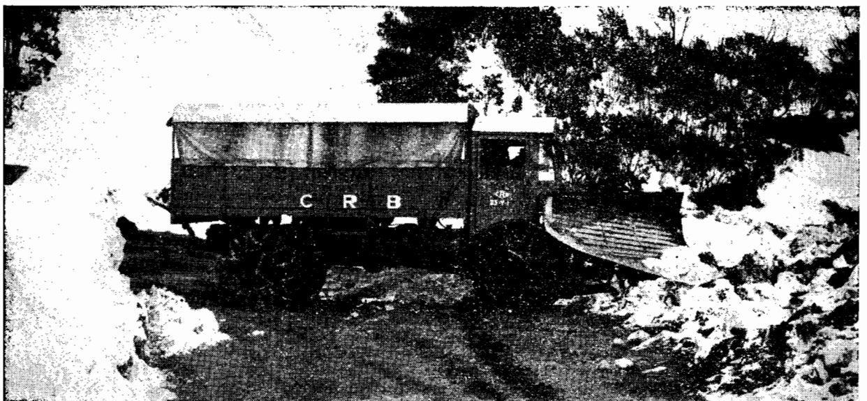
Plate No. 39.—The Matador Snow Plough at Mt. St. Bernard, one of the few turning points on the Alpine Road.
