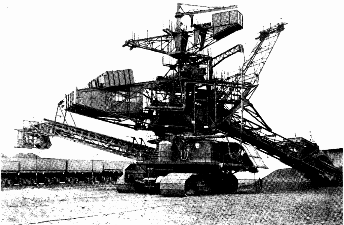
TYPE OF BUCKET WHEEL COAL DREDGER OBTAINED RECENTLY FROM GERMANY AND BEING ERECTED AT YALLOURN OPEN CUT.
