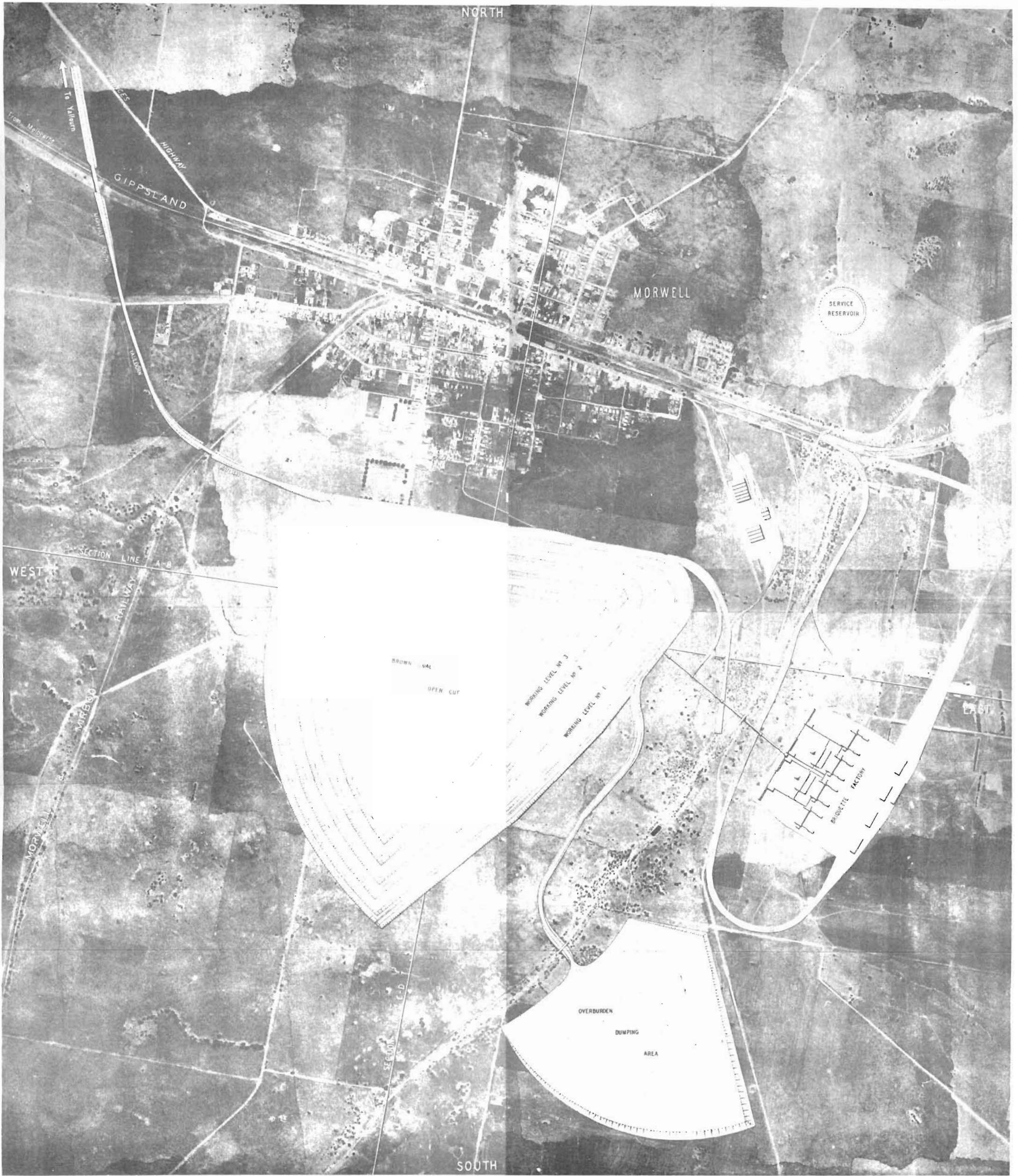
STATE ELECTRICITY COMMISSION OF VICTORIA MARYVALE SOUTH PROJECT PLAN SHOWING POSITION OF OPEN CUT AND BRIQUETTE FACTORY
