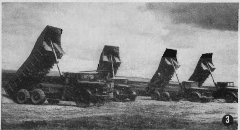
3 10-TON DIESEL TRUCKS USED FOR OVERBURDEN REMOVAL, YALLOURN NORTH OPEN CUT
