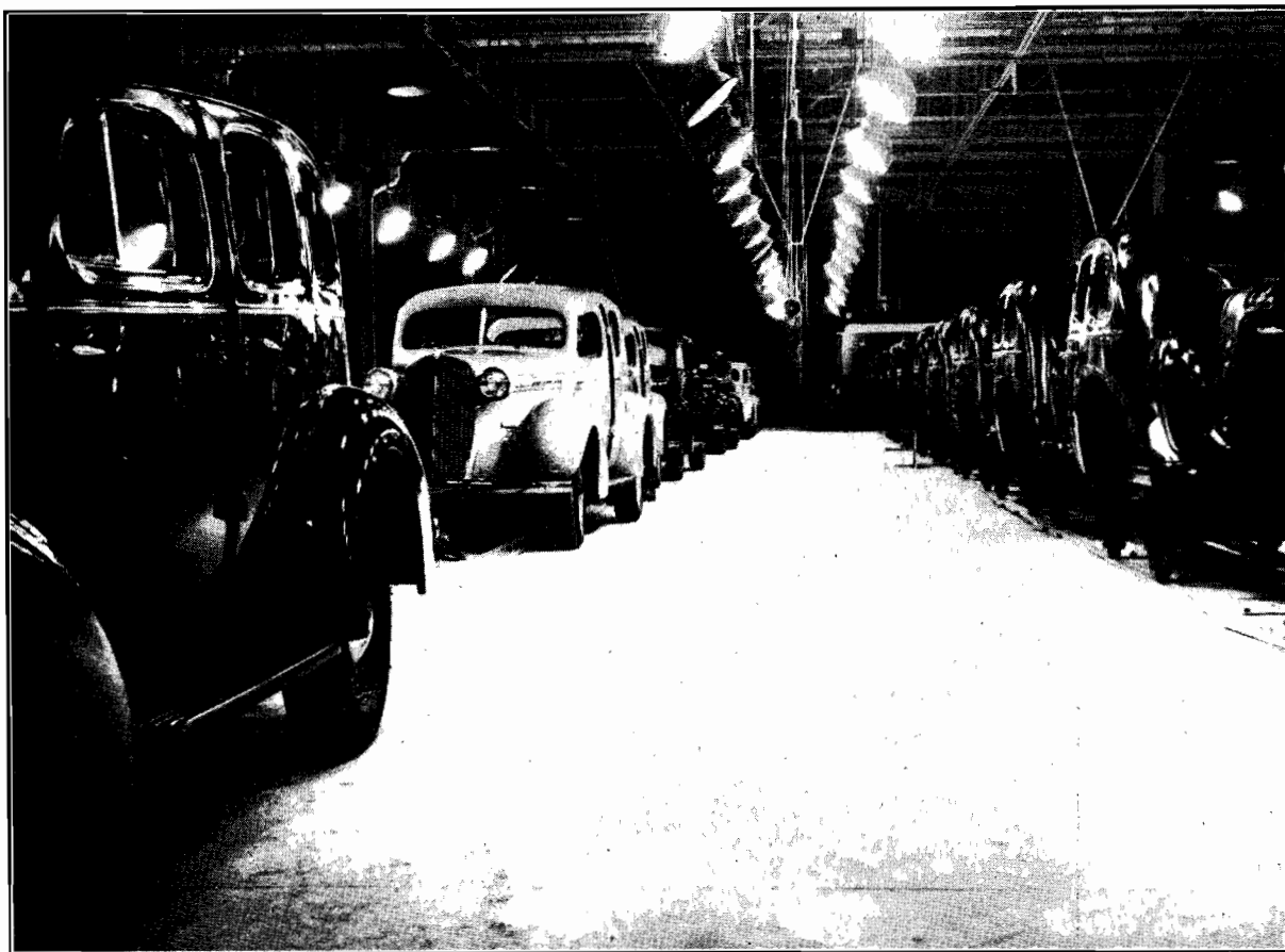
Application of discharge type lamps in a motor assembly plant (Port Melbourne).
