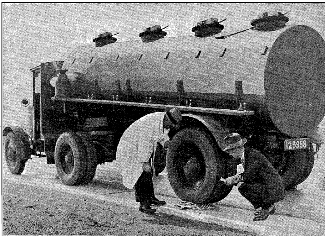
Plate No. 10.—Loadometers in use.
