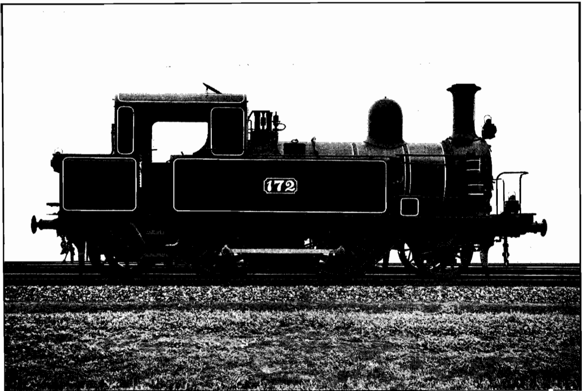
"F" CLASS LOCOMOTIVE ALTERED FOR MOTOR TRAINS.
