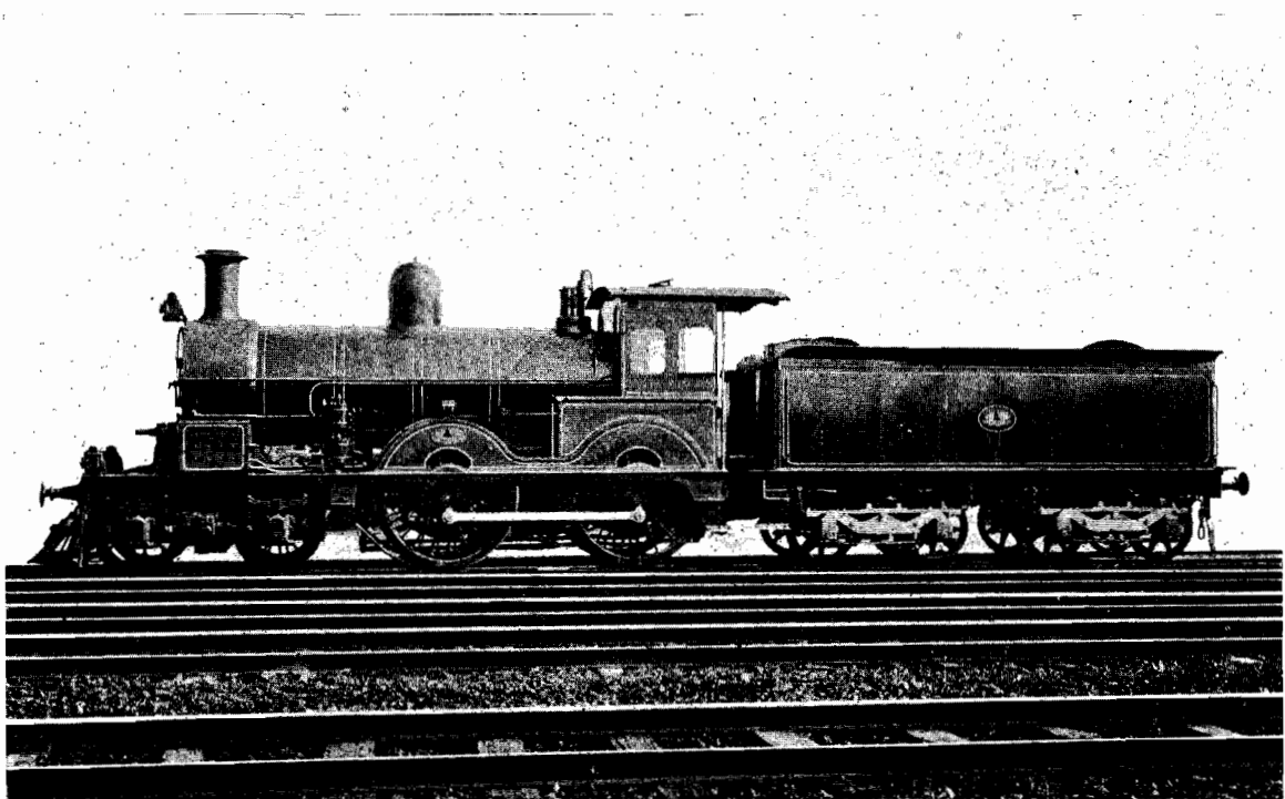
VICTORIAN RAILWAYS. PASSENGER LOCOMOTIVE, "AA" CLASS. (Tractive Power, 20,860 lbs.)
